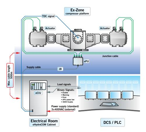
With its clear system interfaces, eHydroCOM is easy to integrate into existing plant control systems.
